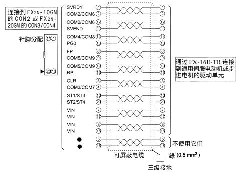
I / 0 电缆 FX-16E-150CAB,FX-16E-300CAB,FX-16E-500CAB,FX-16E-150CAB-R,FX-16E-300CAB-R,FX-16E-500CAB-R
