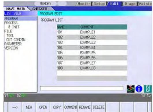
(2) Press the [OPEN] menu key, and input the NC program No. to be read out.
