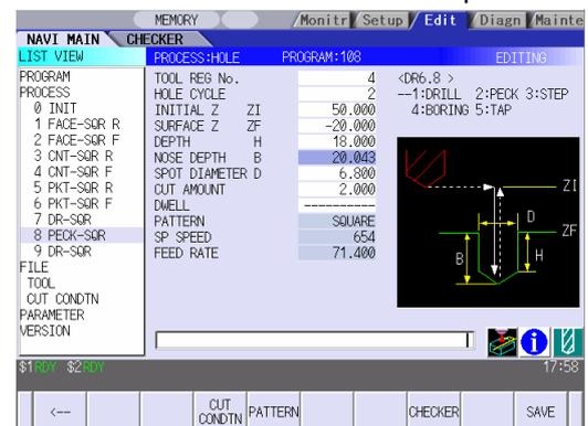
**(Note 1)** The contents in the data setting area are only displayed when [INPUT] key is not pressed and will be invalidated if the screen is changed at this time. Data for the currently selected setting item will be set when [INPUT] key is pressed.
