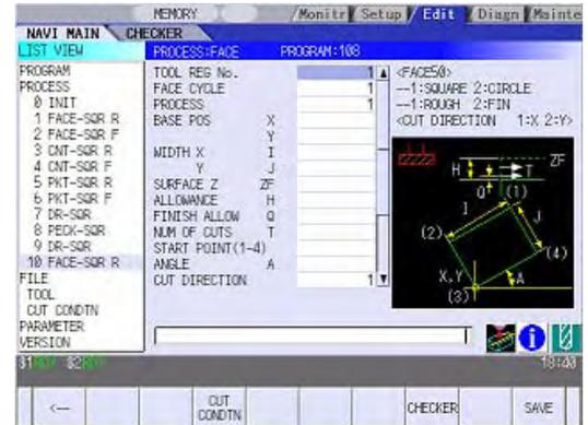
**(Note)** If the [←] menu key is pressed during adding the process, the screen will return to the state before pressing the [NEW] menu key (state of the 1).
