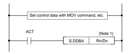
(Note 1) The file registers (Rn) and data registers (Dn) in the range usable by the user can be used in the control data buffer of the asynchronous type DDB. The file registers (R) usable by the user are from R4000 to R4499 (not backup) and from R6400 to R7199 (backup).
