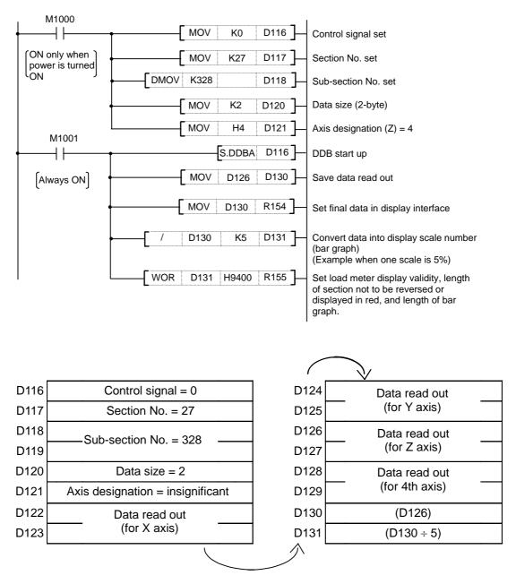
In this example, only the Z axis data is read out, and the previous states are held for the X, Y and 4th axis data.
