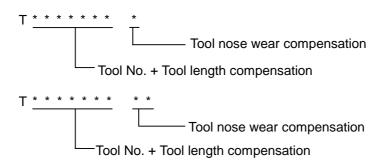
In this case, the tool length compensation No. is the last two digits of the high-order digit.
