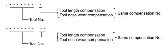
(b) When designating the tool length compensation No. and tool nose wear compensation No. independently.
