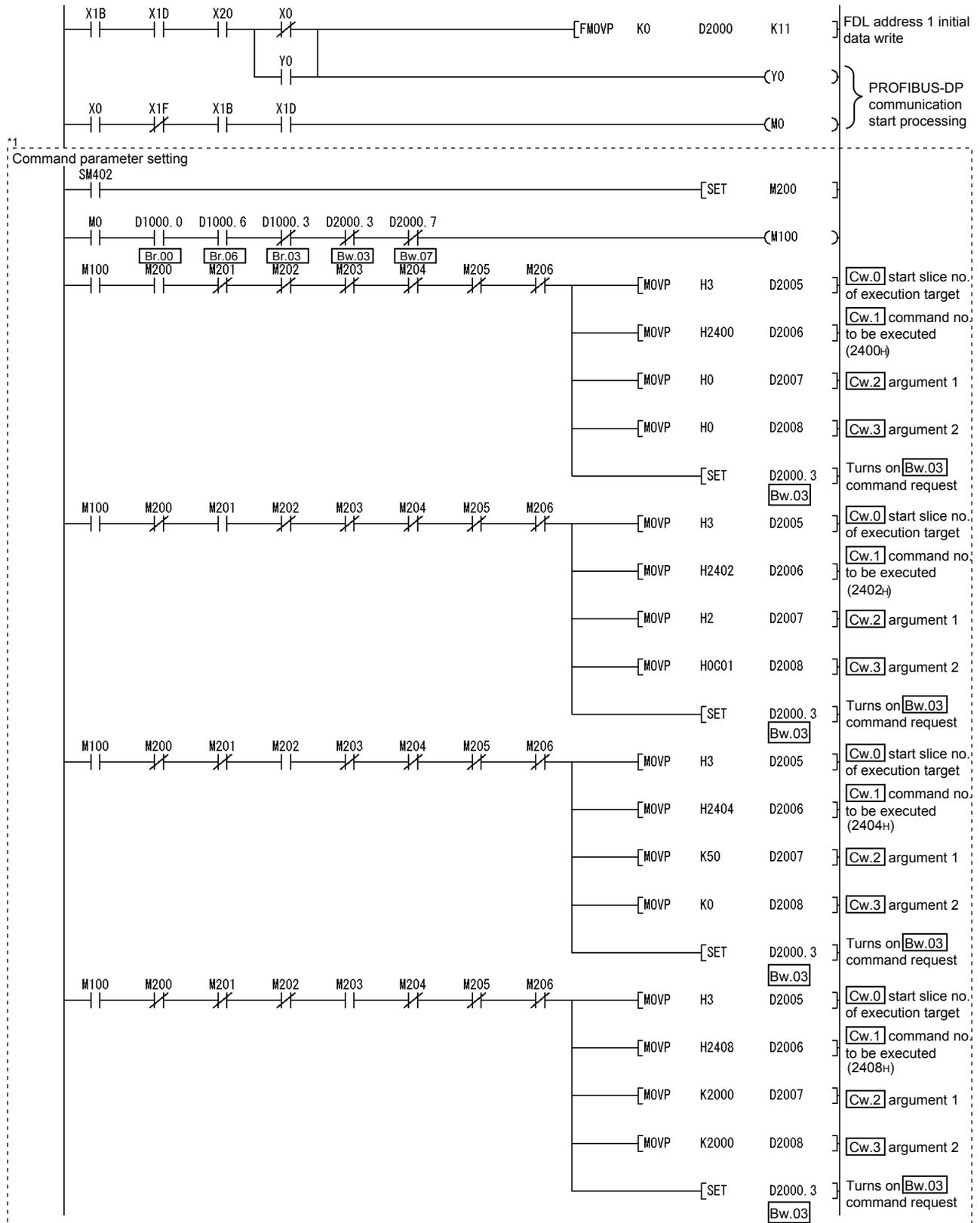
\*1 The program area enclosed by the dotted line is not required when GX Configurator-ST is used to set the command parameters.
