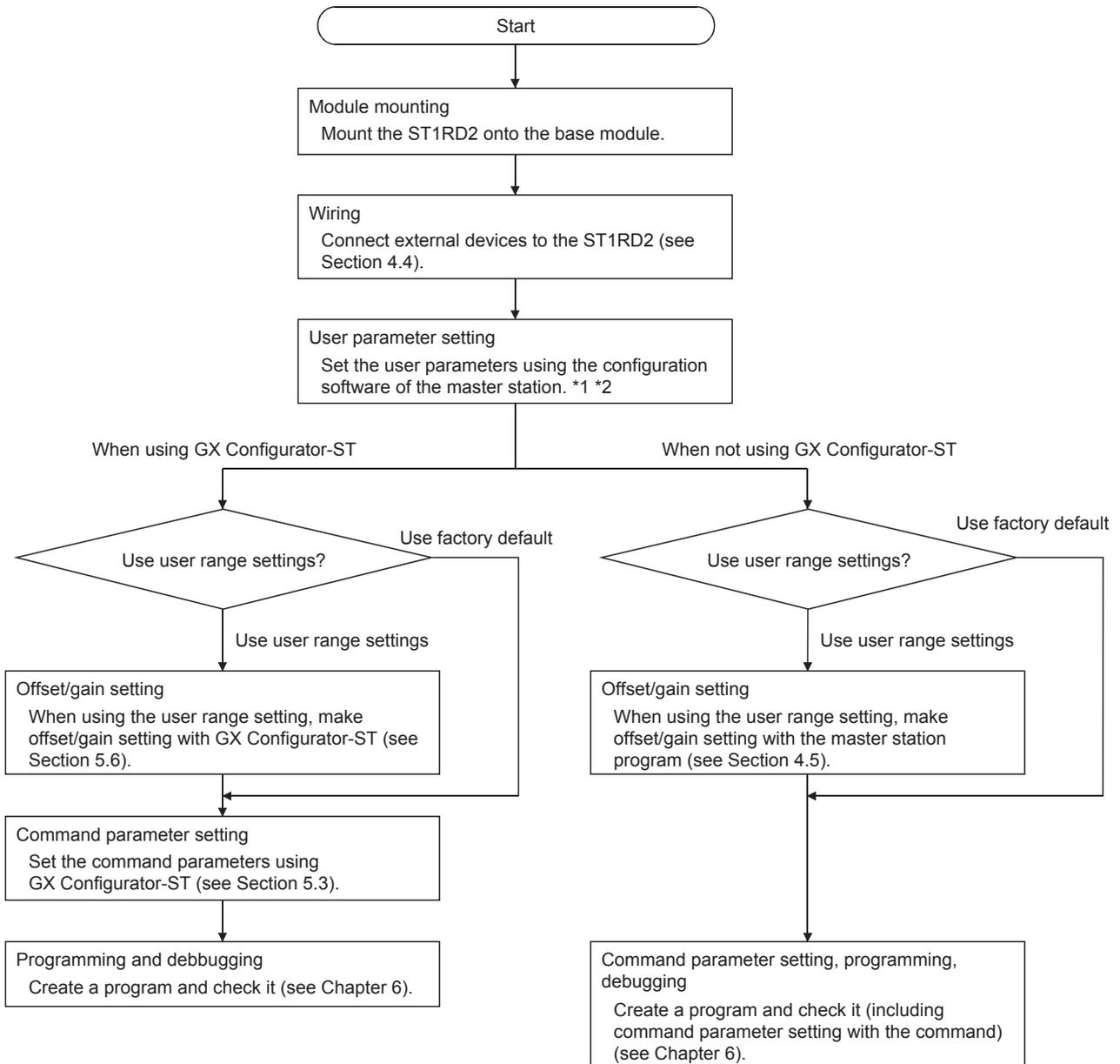
\*1 When using the user range setting, set the offset/gain value selection (user parameter) as "user range setting".
