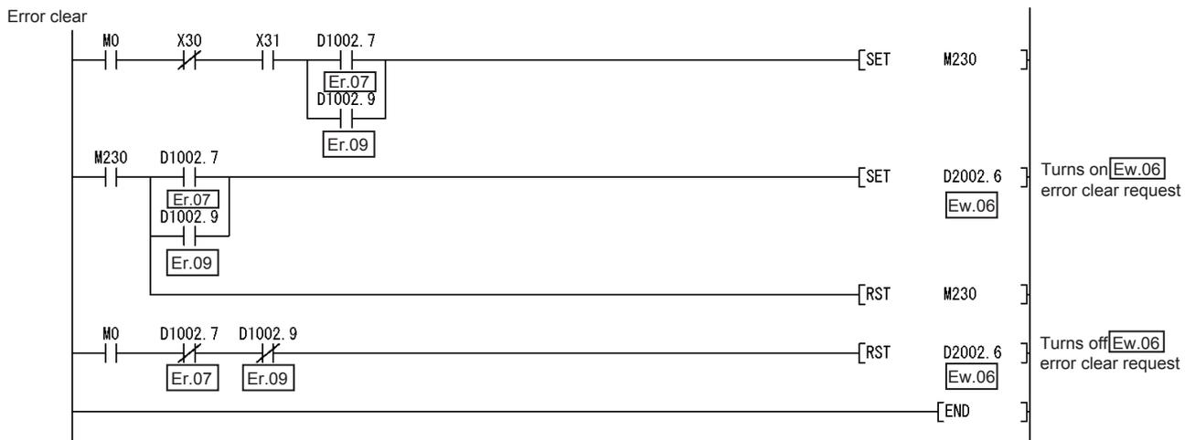
6.3 When Using AJ71PB92D/A1SJ71PB92D as Master Station
