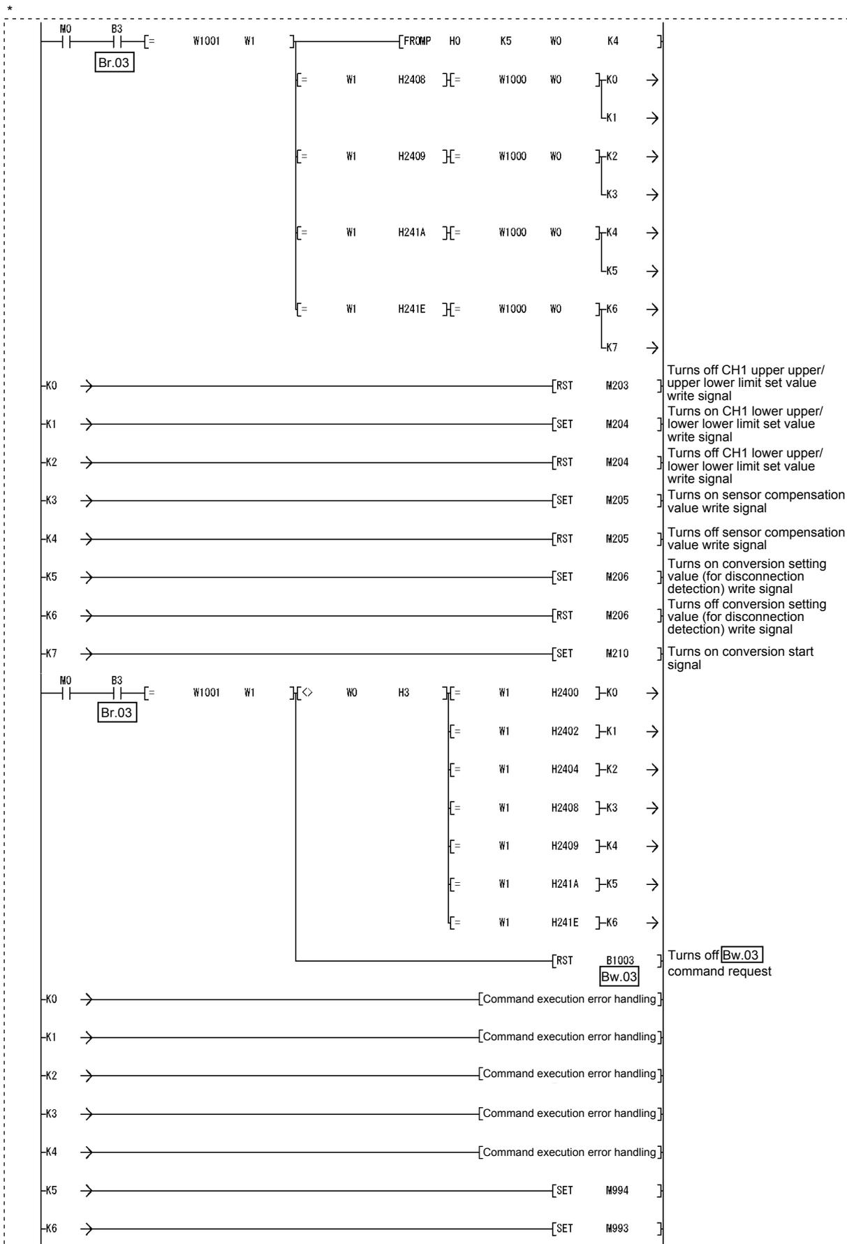
\* The program area enclosed by the dotted line is not required when GX Configurator-ST is used to set the command parameters.
