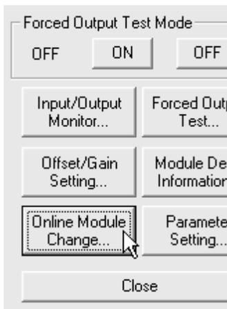
2) Click the **Online Module Change** button on the "System Monitor" screen. Then, confirm that the RUN LED of the selected ST1RD2 is flashing at 0.25s intervals.
