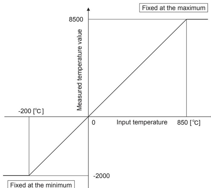
Figure 3.1 Conversion characteristic of -200 to 850°C range
