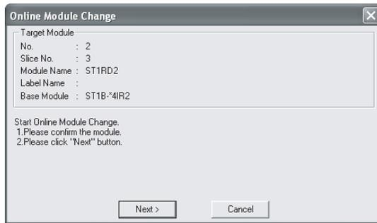
3) Confirm that the ST1RD2 displayed as "Target Module" is the ST1RD2 to be replaced and click the **Next** button.
