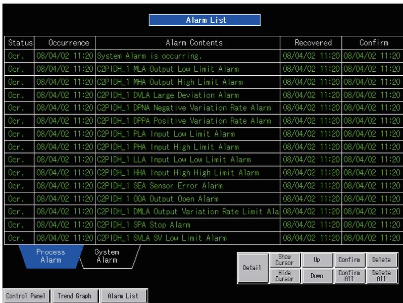
The screenshot shows the 'Alarm List' screen with a table of alarm occurrences. The table has columns for Status, Occurrence, Alarm Contents, Recovered, and Confirm. Below the table are buttons for 'Process Alarm' and 'System Alarm', and a control panel with buttons for 'Detail', 'Show Cursor', 'Up', 'Confirm', 'Delete', 'Hide Cursor', 'Down', 'Confirm All', and 'Delete All'. A navigation bar at the bottom includes 'Control Panel', 'Trend Graph', and 'Alarm List'.
