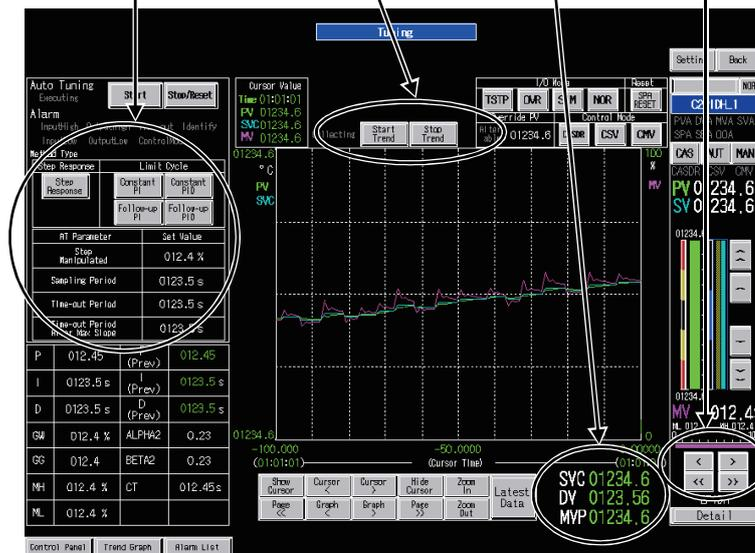
The two type screens have same parts in functionality. However, positions of the auto tuning switches, trend start/stop switches, and MV increase/decrease switches in a faceplate; and display position of the internal parameters such as SVC/DV/MVP slightly differ so that they can be easily pressed.
