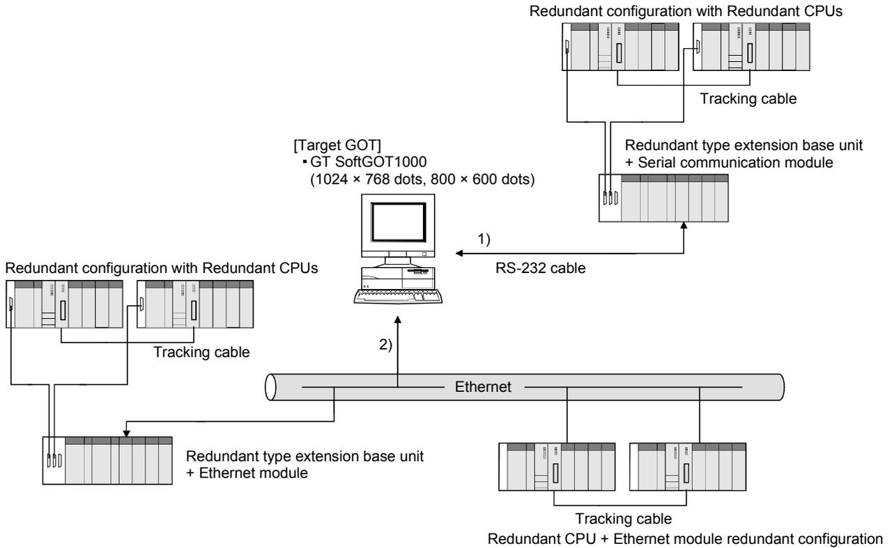
[Paths connectable to the Redundant CPU]
