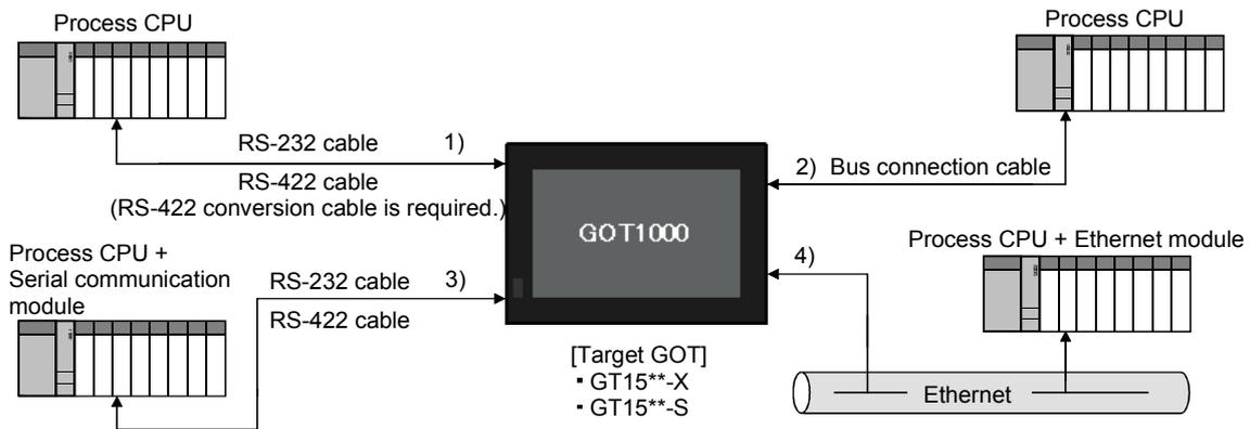
[Paths connectable to the Process CPU]
