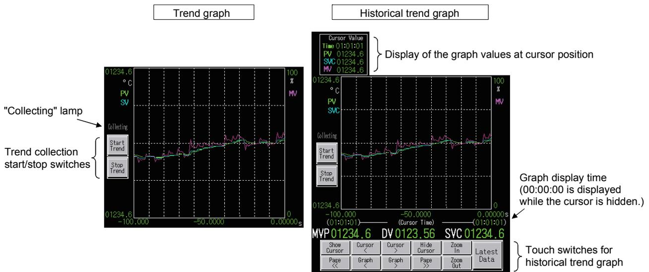
Compared to the trend graph, the historical trend graph has touch switch function that displays/deletes/moves the cursor and display function that displays graph values at the cursor position. For details of touch switches for historical trend graph, refer to "GT Designer2 Version 2 Screen Design Manual (For GOT1000 Series)".
