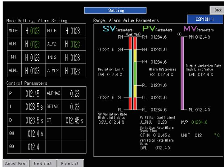
Touching the "Back" switch at the top right of the screen returns the display to the previous screen.
