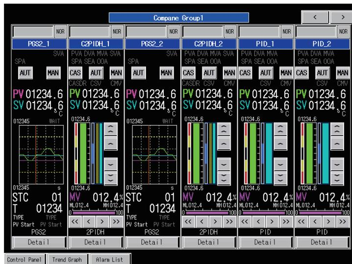
Operation monitoring using lamps and switches on a faceplate is possible. The "<" and ">" switches at the top right of the screen can switch the pages. The "Detail" switch on a faceplate can switch the display to the tuning screen corresponding to each tag.
