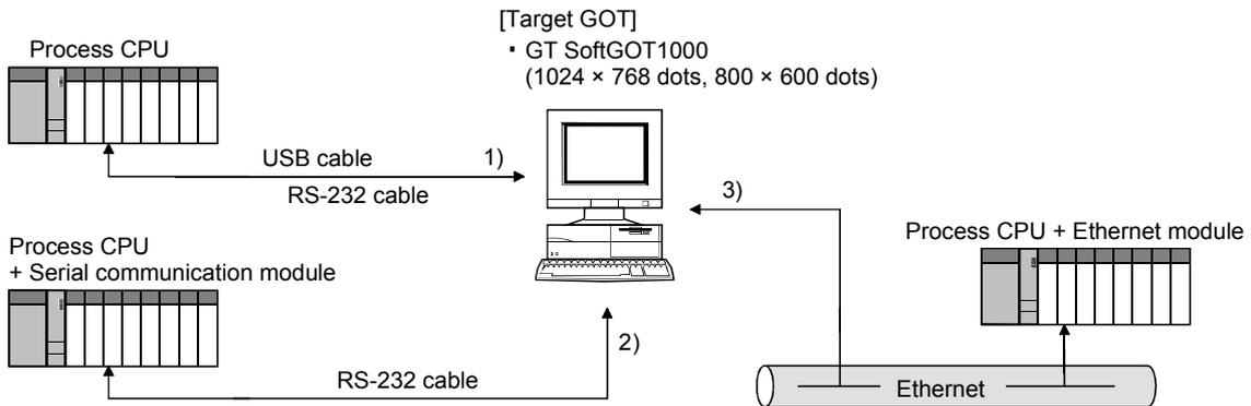
[Paths connectable to the Process CPU]
