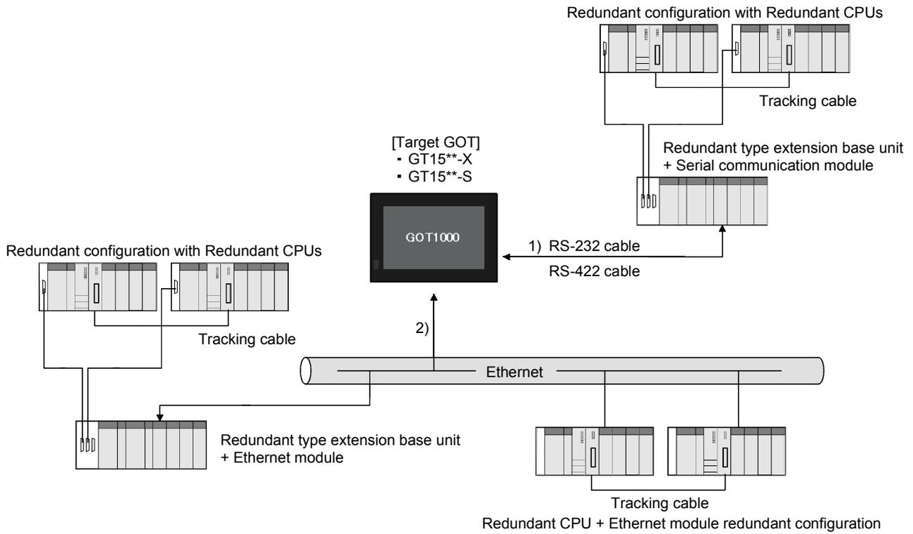
[Paths connectable to the Redundant CPU]
