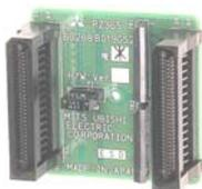
This interface is required to use the robot arm's hand output signals. This interface is pre-installed on the controller.
