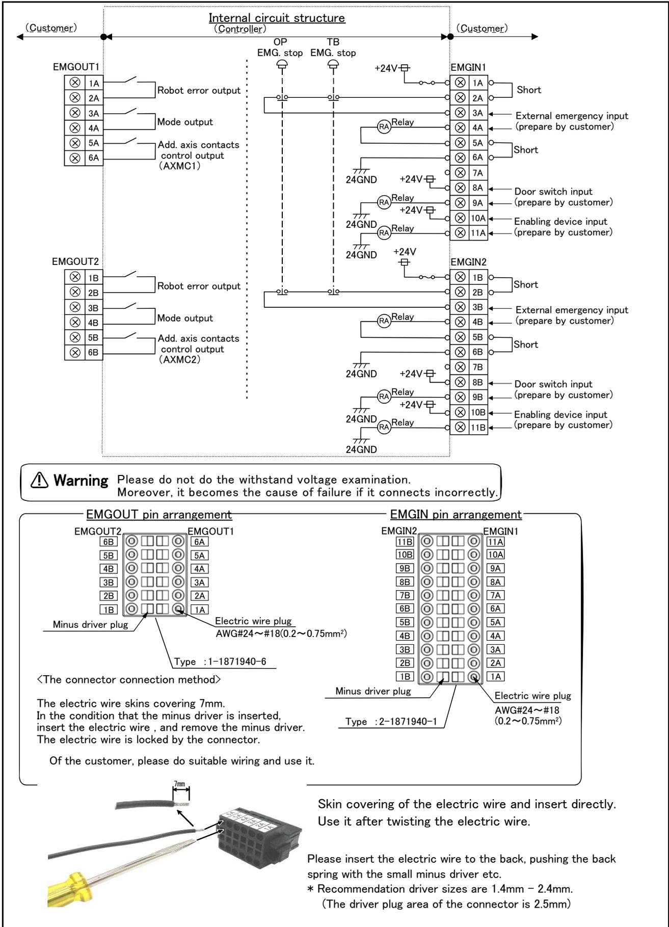
Fig.3-10 : External emergency stop connection
