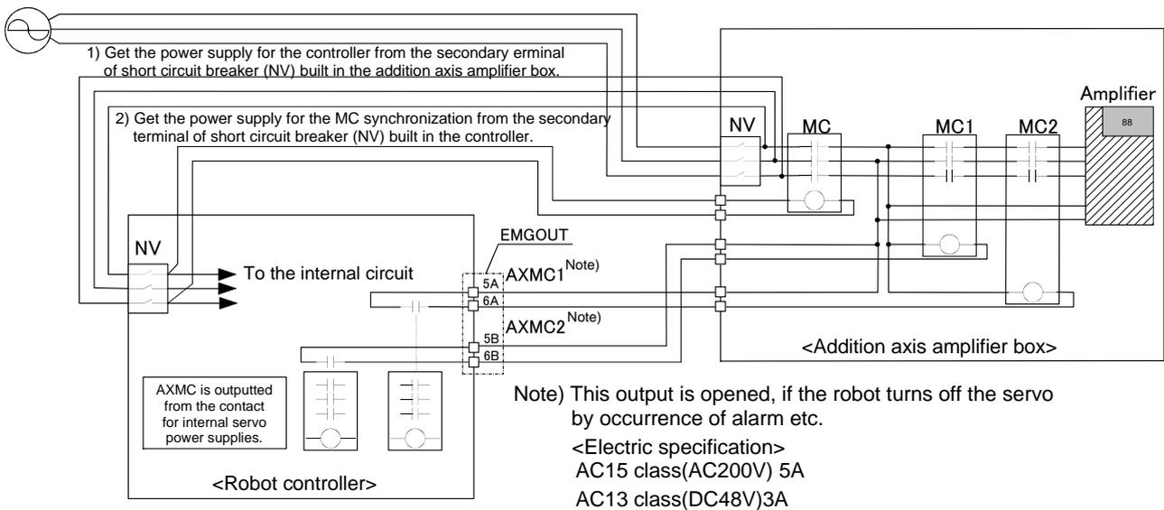
Fig.3-14 : Example of circuit for addition axes of Magnet contactor control output
