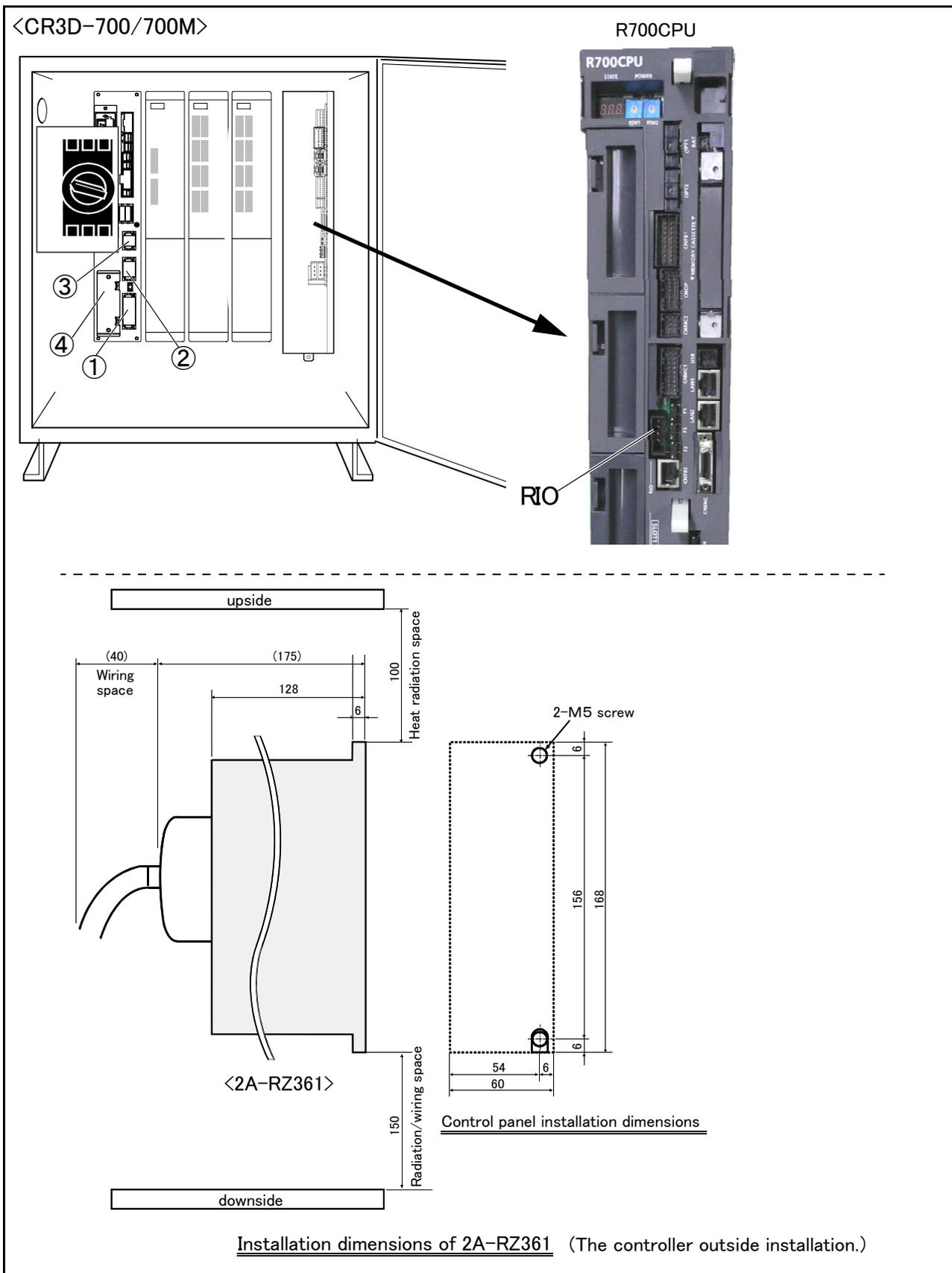
Fig.3-23 : Installing the parallel I/O unit (CR3D-700/700M)
