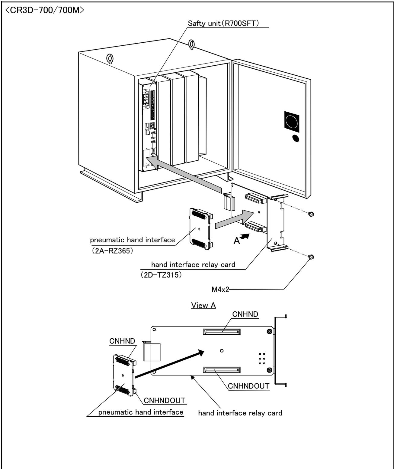
Fig.3-18 : Installation of the pneumatic hand interface (CR3D-700/700M)
