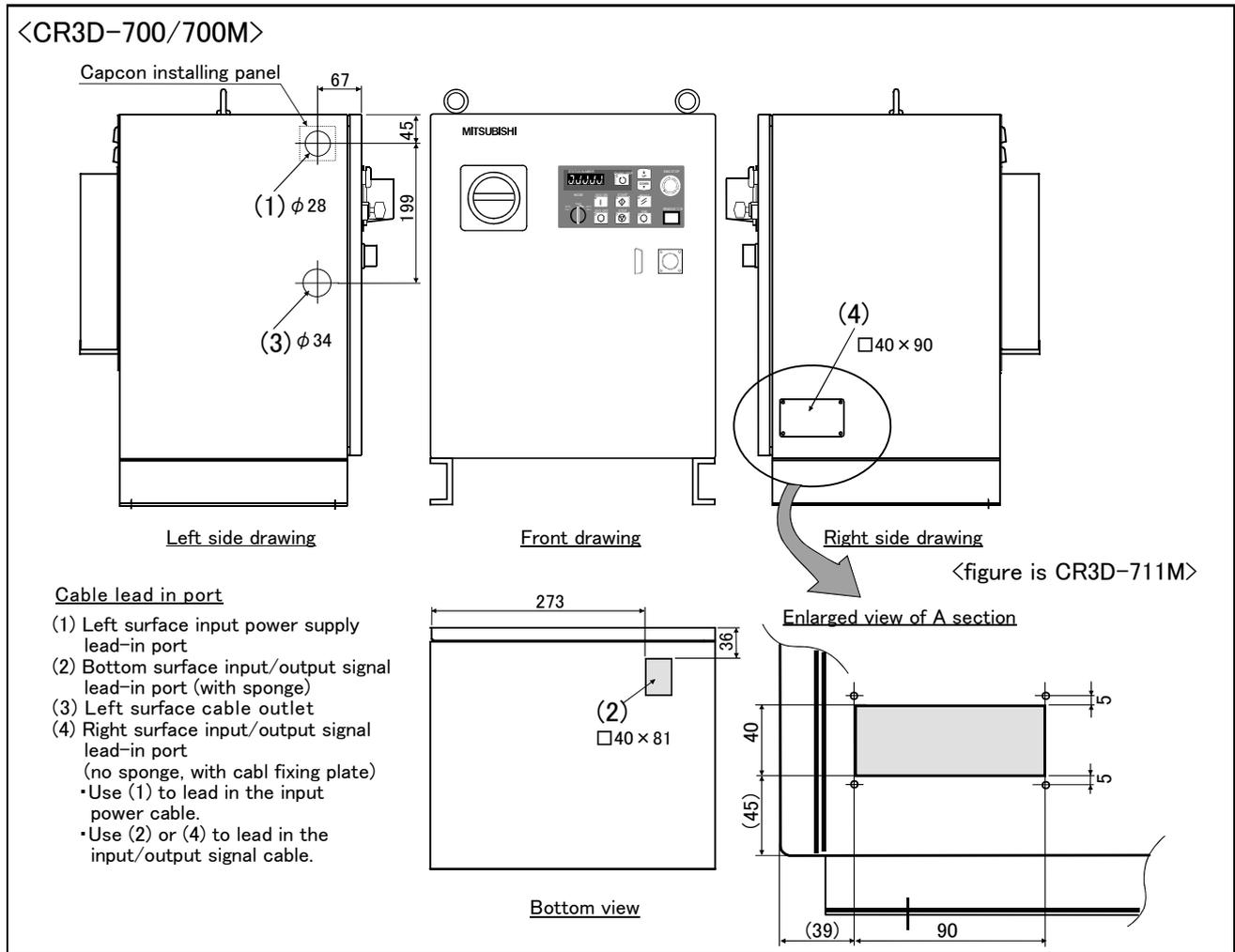
☒ 3-8 : Cable lead-in and dimension of the controller (CR3D-700/700M)
