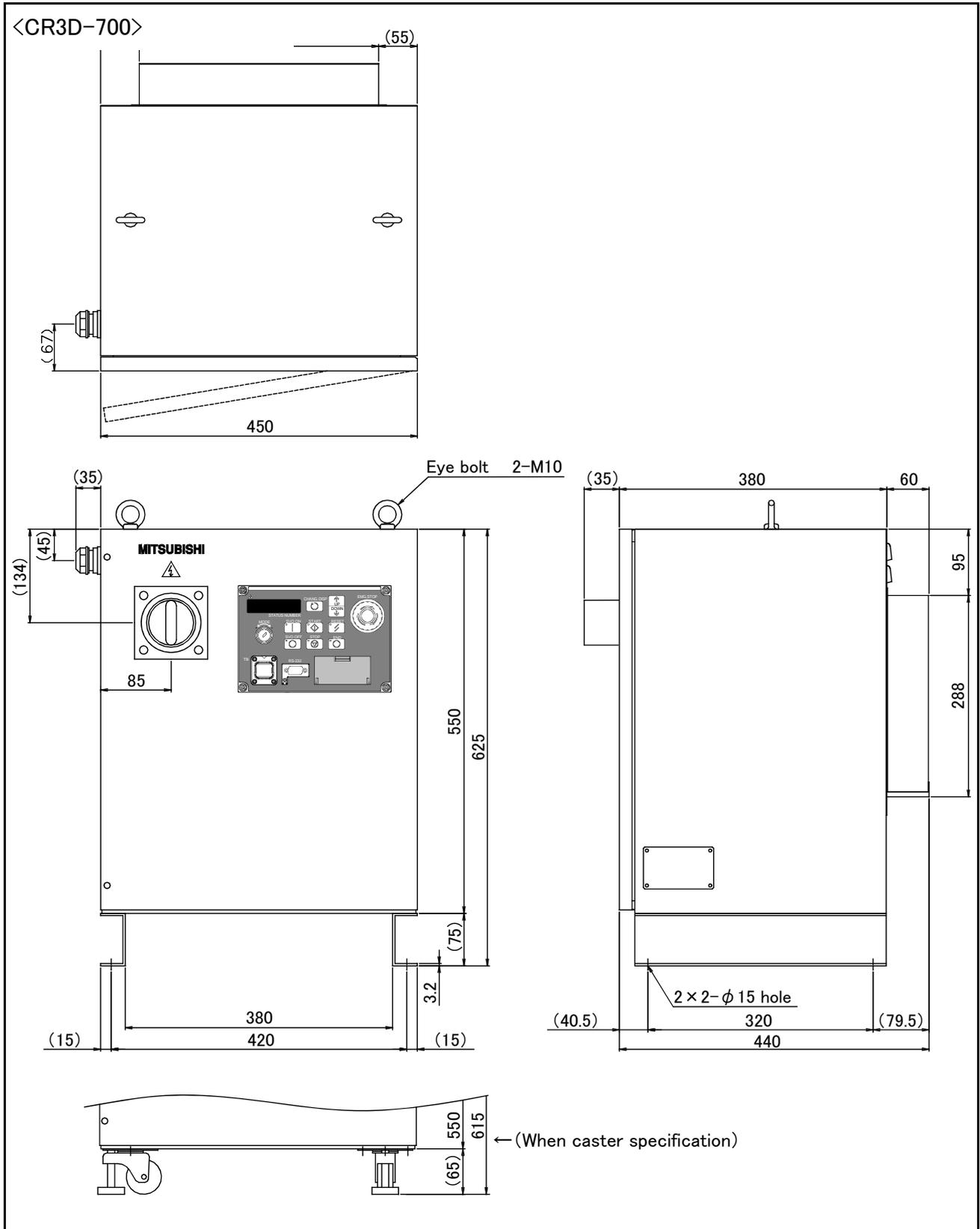
图 3-4 : Outside dimensions of controller(CR3D-700)
