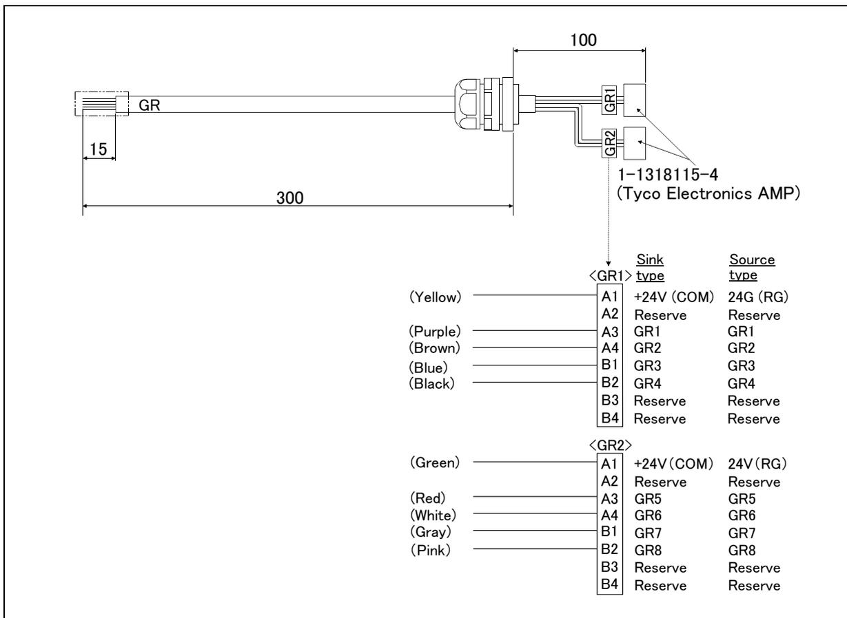
Fig.2-12 : Outline dimensional drawing and pin assignment
