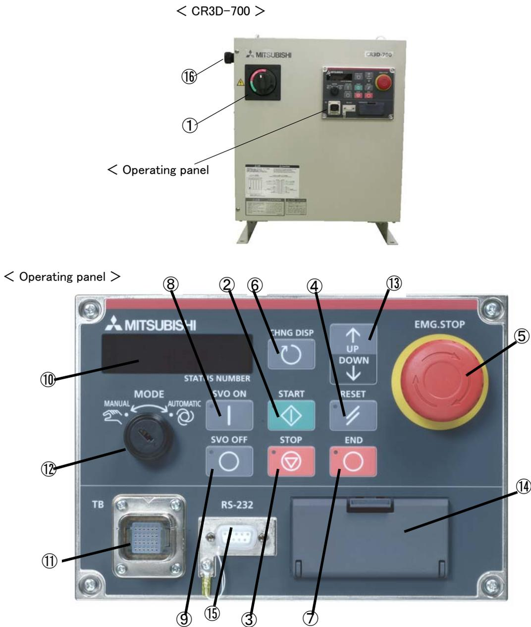
Fig.3-1 : Names of controller parts
