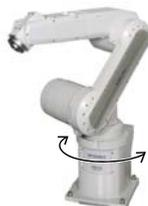
The J1 axis operating range is limited by the robot arm's mechanical stopper and the controller parameters.
