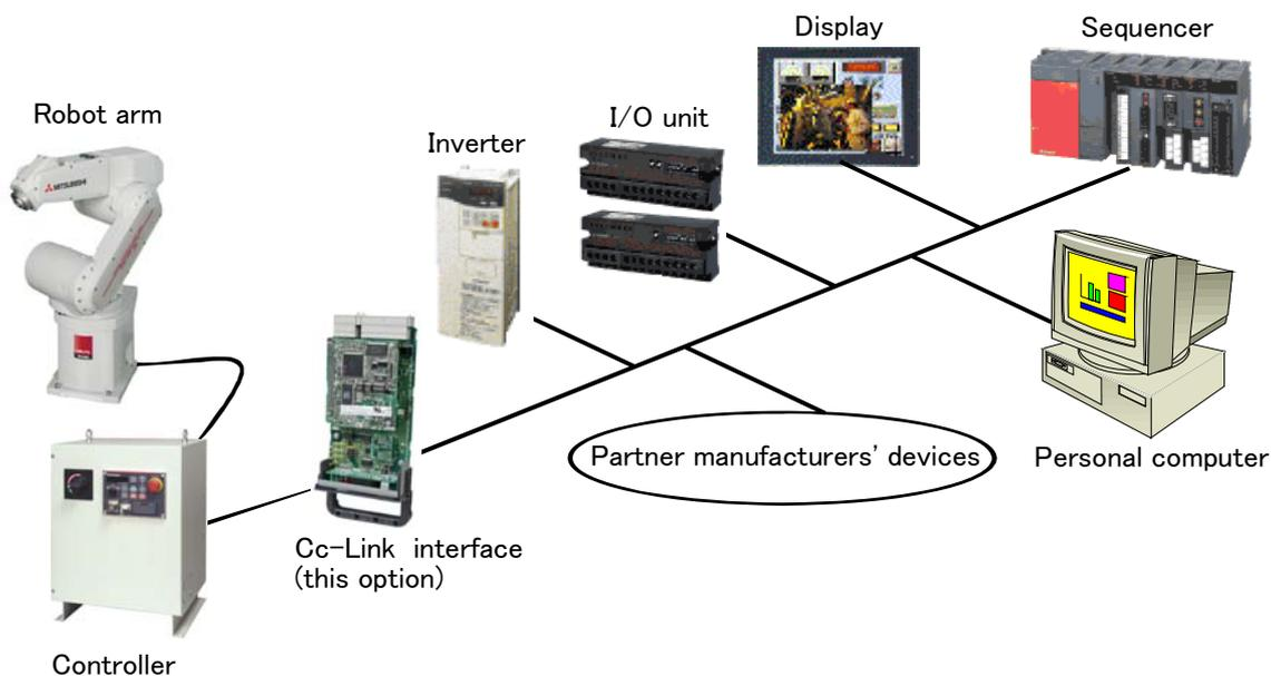
Fig.3-28 : Example of CC-Link Product Configuration
