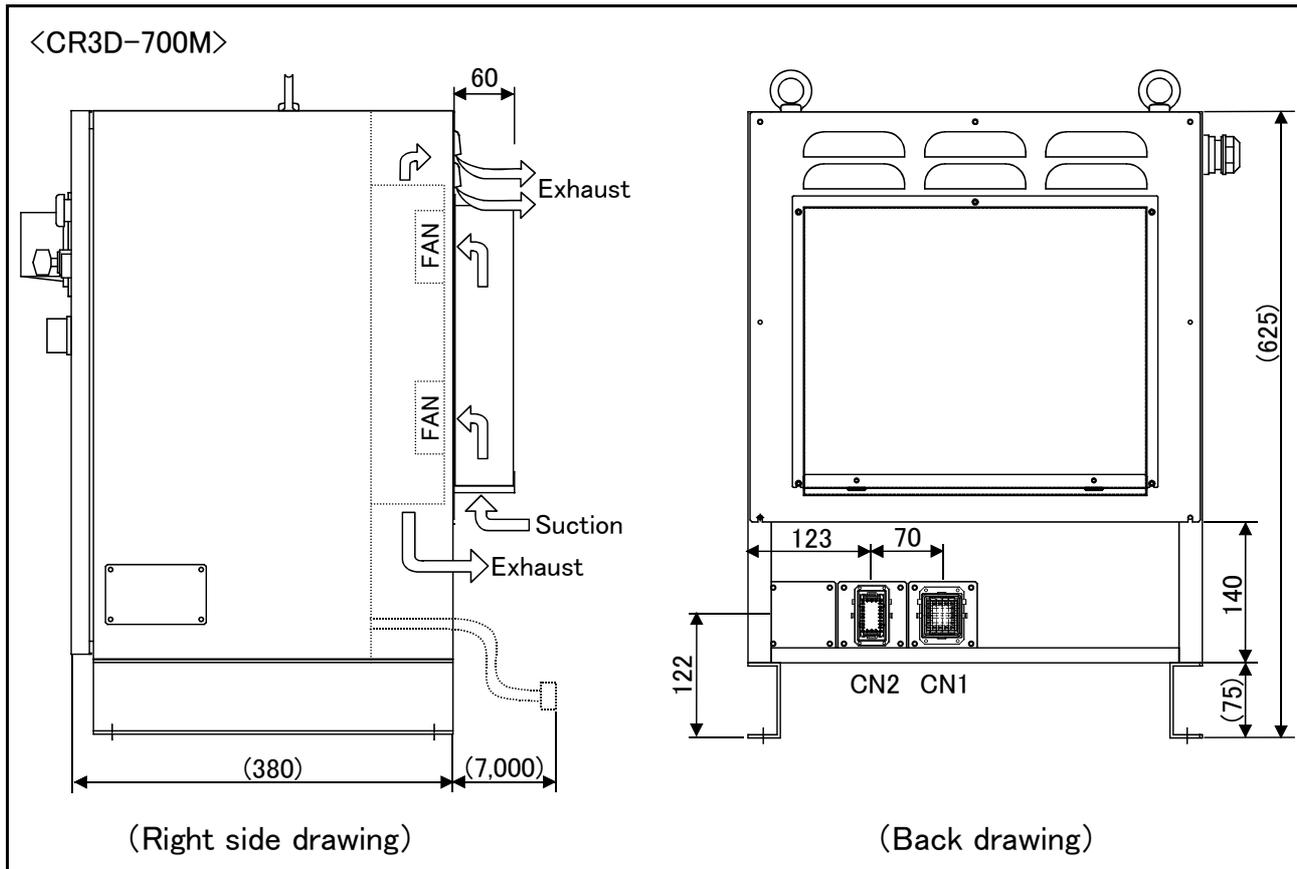
Fig.3-5 : Outside dimensions of controller (CR3D-700M Supplement)
