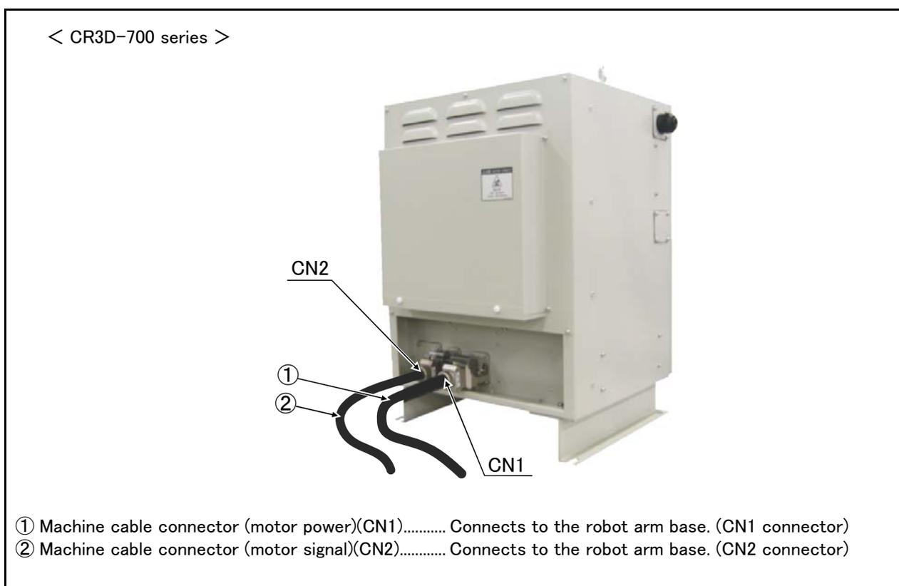
Fig.3-2 : Names of each part (Rear side CR3D-700 series)
