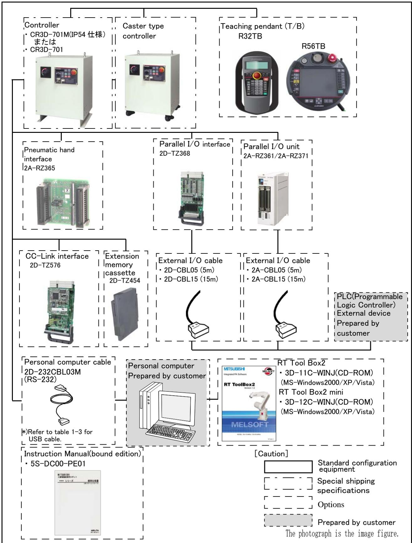
Fig.1-1 : Structural equipment
