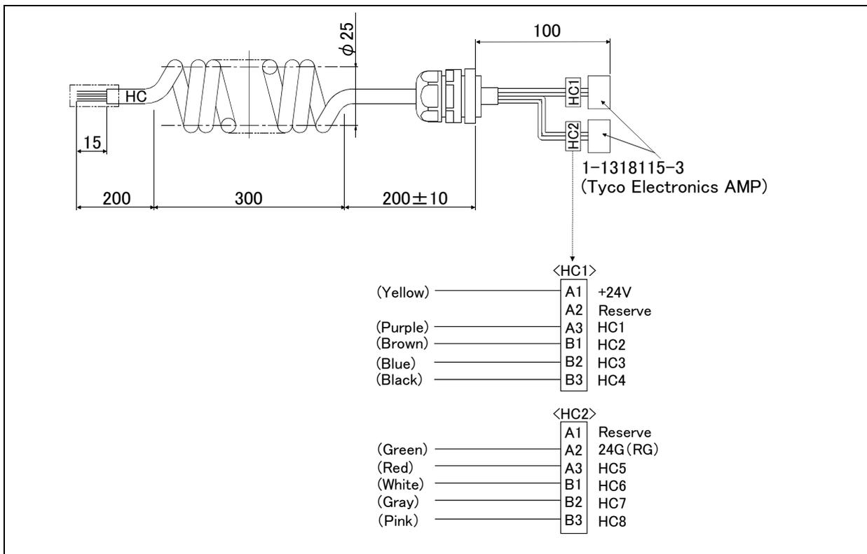
Fig.2-11 : Outside dimensional drawing and pin assignment
