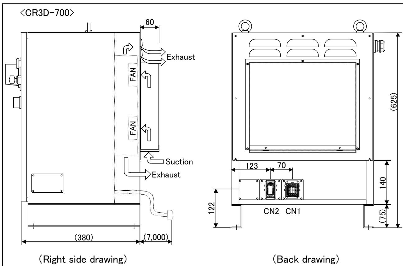
Fig. 3-6 : Outside dimensions of controller (CR3D-700 Supplement)
