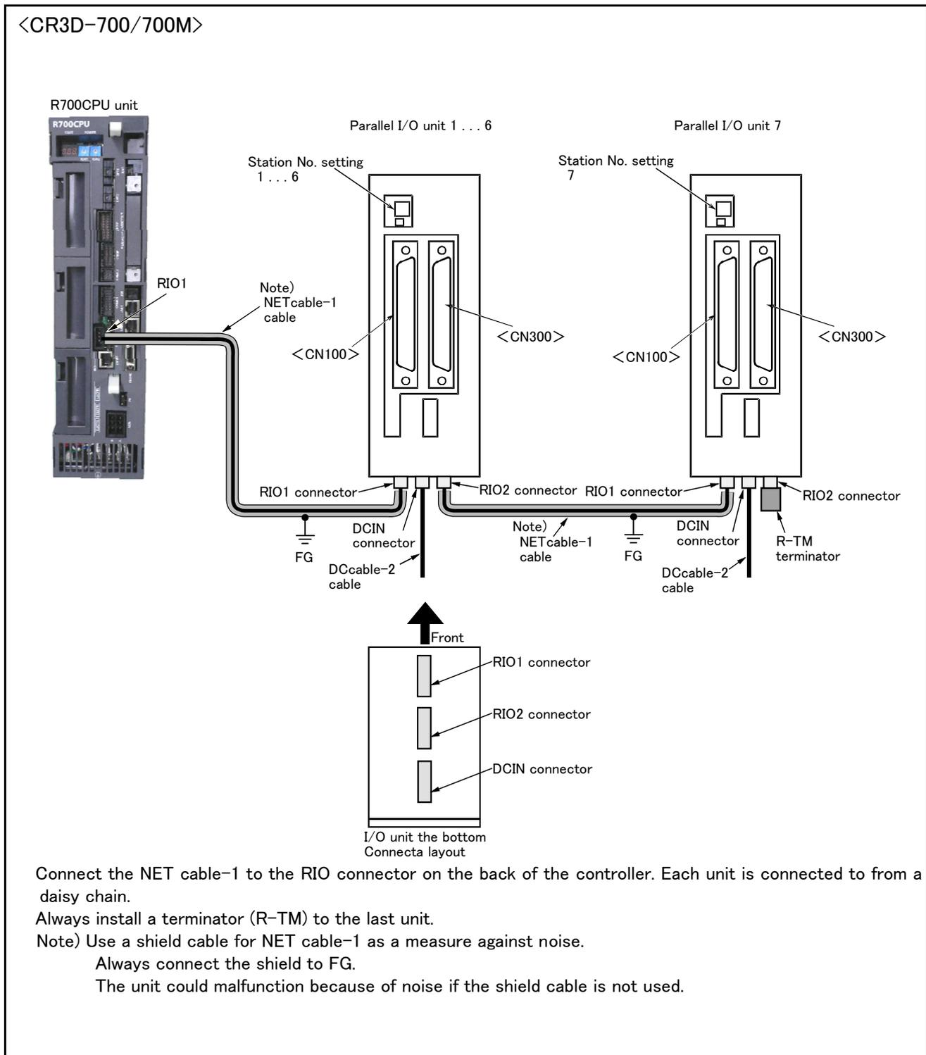
Fig.3-24 : Connection method of expansion parallel I/O unit (CR3D-700/700M)
