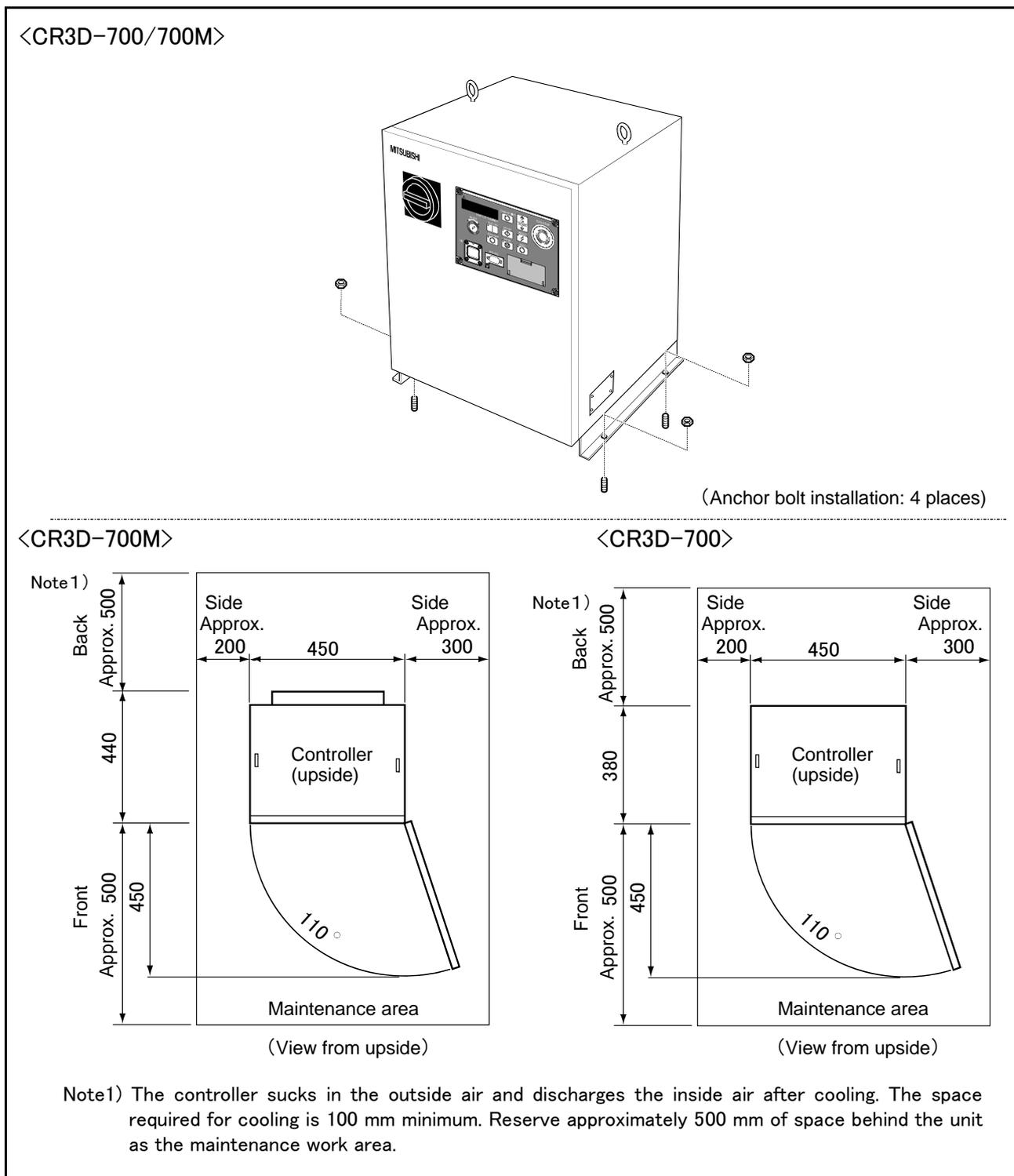
Fig.3-7 : Installation of controller (CR3D-700/700M)
