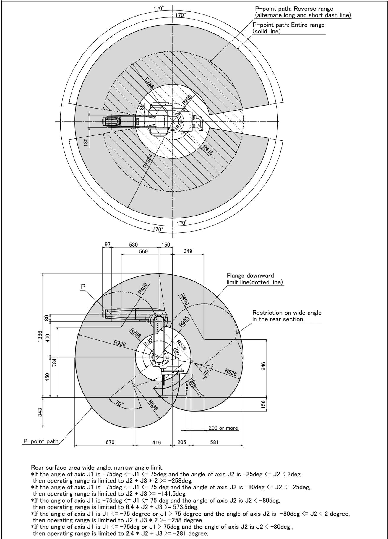
Fig.2-4 : Operating range diagram : RV-12SD/12SDC
