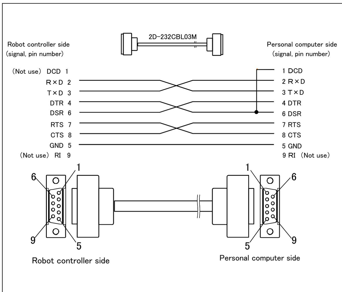
Fig.3-27 : Personal computer cable connection
