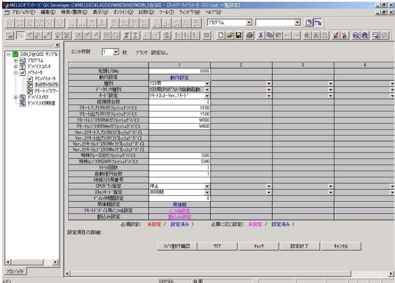
(2) Set the automatic refresh parameters using the following procedure.
